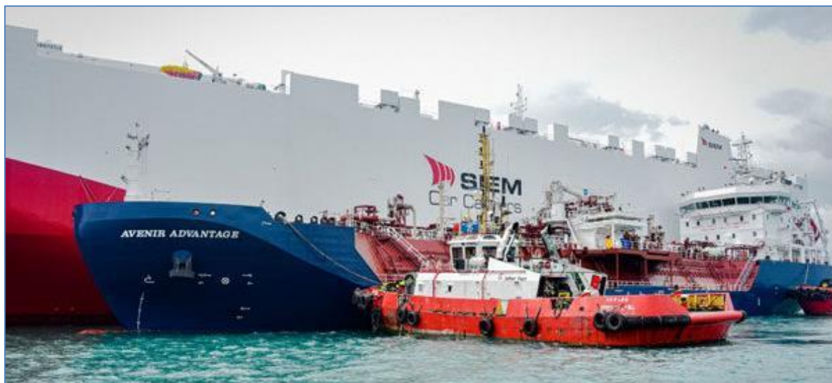
Figure 7 Berthing of the LNG bunker ship onto a commercial ship
