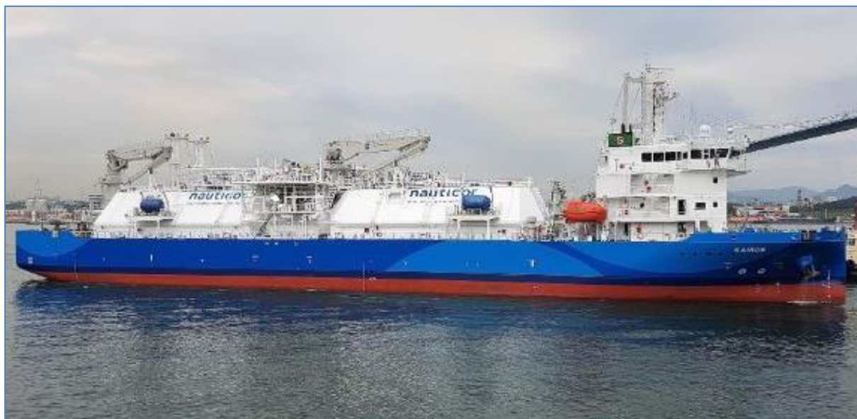
Figure 9 Fenders and cranes on the LNG bunker ship
