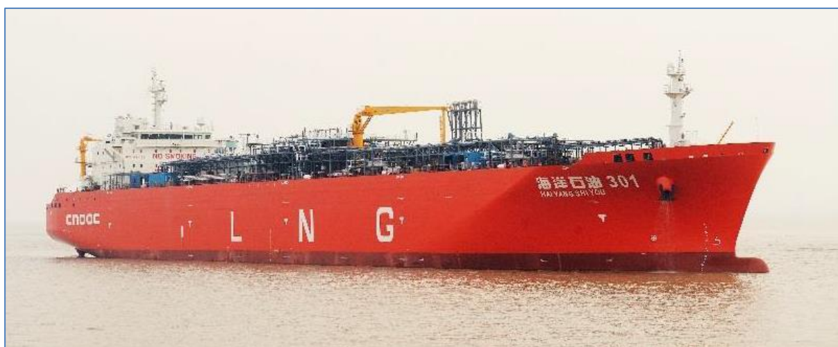
Figure 17 LNG feeder ship with a capacity of 30,000 m 3
