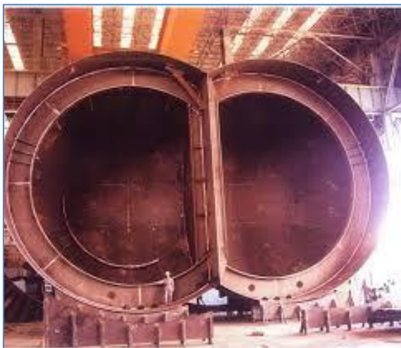
Figure 16 IMO "C" type cargo tank of the „Bilobe“ type
