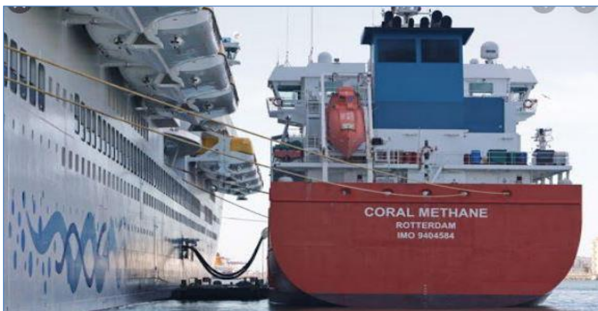
Figure 8 Supplying fuel to a cruise ship from a LNG bunker ship with a capacity of 7,500 m 3
